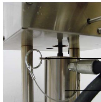
Manifold Block (#170-20) Safety Pin (#171-23-1)
