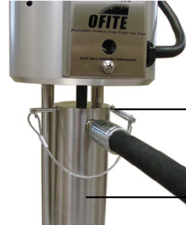
Manifold Block (#170-20) Safety Pin (#171-23-1)
