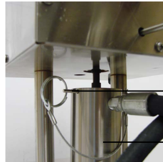
Manifold Block (#170-20) Safety Pin (#171-23-1)
