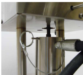
Retainer Pin with Lanyard
